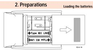
Fig. 2: Position of batteries
